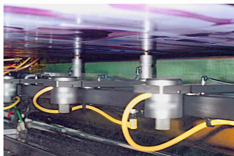
ABD register-nozzle bar stretching the web width by non-contact air pressure
